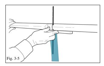
**NOTE:** A good way to ensure that where the rear and front molding meet between the doors align vertically is to hold a plastic straight edge against the bottom of the front molding and use it as a guide for the rear molding as shown in Fig. 3-5. Tolerance for alignment in the vertical direction of the front and rear molding in relation to each other is 0.0mm +/-1.0mm.
